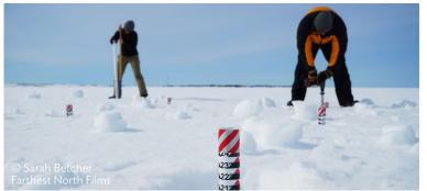
On ice measurements Ikaagvik Sikukun measures sea ice growth and melt over the winter and spring, and tracks snow depth.
