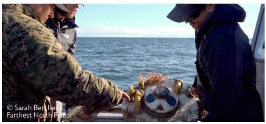
**Ocean mooring** Ikaagvik Sikukun tethered a mooring (science instrument attached to a buoy) in the Sound to measure water temperature.
